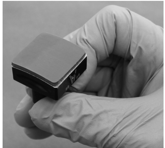
Figure 6: SBR Sensor Without Wear Line (Note: There may be a "sanding line" that remains after sanding is completed, as seen below.)
