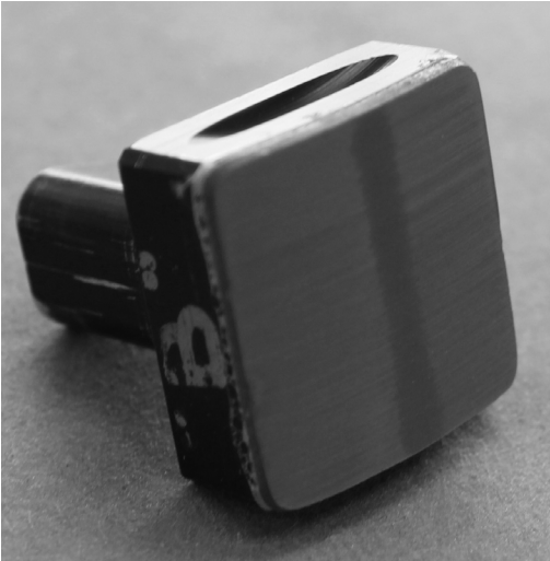
Figure 5: SBR Sensor With Wear Line
